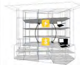
INTERNAL CAP & TRADE EACH TENANT HAS AN ENERGY BUDGET; UNUSED ENERGY CAN BE TRANSFERRED
